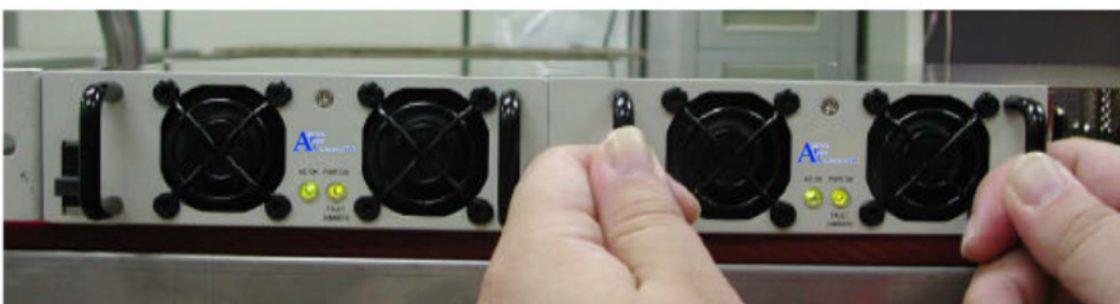
Step 3 : Push to fully contacted and PWR OK LED is ON.
